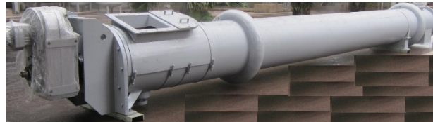
Picture 4.1a. The industrial bottom slag cooling equipment used for experiment
