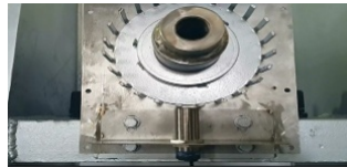
Figure 3.5: Image of structure of installing sensor for measuring rotary velocity of axis
