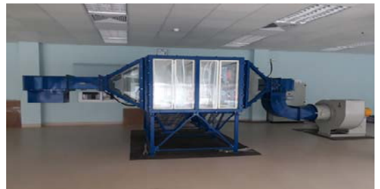
Figure 3.1. Physical model of electric dust filter for experiment
