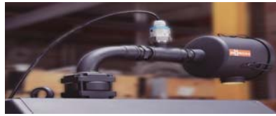
Figure 3.10. Pressure measuring device Cerabar PMC131 Figure 3.12. Temperature measurement device TSM187
