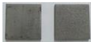
Figure 3.3. C45 steel sample before and after spray cleaning to create roughness
