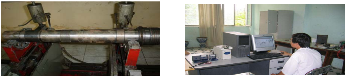
Fig. 14. Some pictures of measuring process defining specific vibration of the spindle
