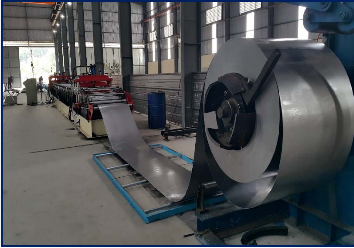
Roll forming machine to fabricate CE electrodes
