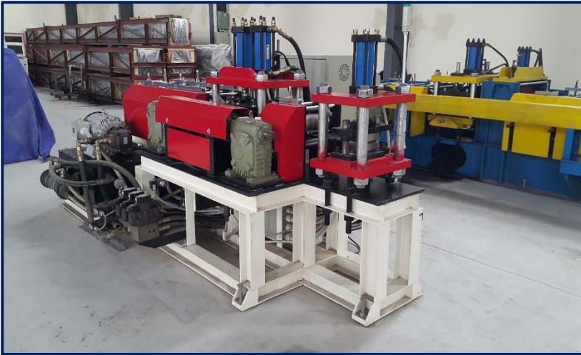
Servo-controlled punching machine to fabricate Discharge electrodes
