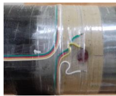
Figure 4.5 Circuit of Wheatstone bridge and tenzo pasted on the shaft
