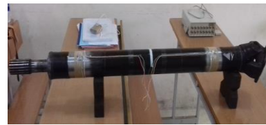
Figure 4.5 Circuit of Wheatstone bridge and tenzo pasted on the shaft
