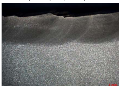
M7: I_h = 8,5kA ; F = 1,7kN ; V_h = 2,0cm/s
