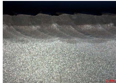
M2: I_h = 6,5kA ; F = 2,0kN ; V_h = 1,75cm/s
