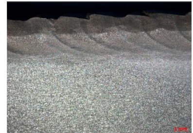
M3: I_h = 6,5kA ; F = 2,3kN ; V_h = 2,0cm/s
