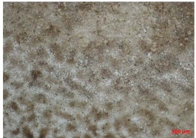
M7: I_h = 8,5kA ; F = 1,7kN ; V_h = 2,0cm/s
