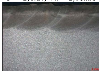
M8: I_h = 8,5kA ; F = 2,0kN ; V_h = 1,5cm/s
