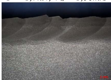
M4: I_h = 7,5kA ; F = 1,7kN ; V_h = 1,75cm/s
