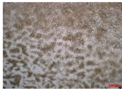
M2: I_h = 6,5kA ; F = 2,0kN ; V_h = 1,75cm/s
