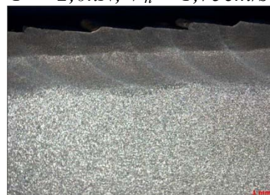
M5: I_h = 7,5kA ; F = 2,0kN ; V_h = 2,0cm/s
