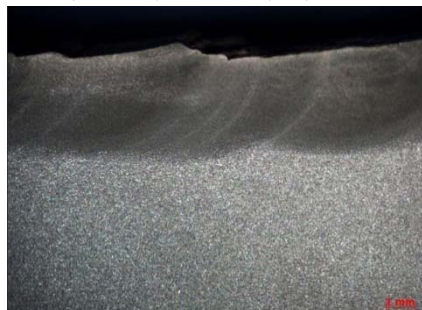
M7: I_h=8.5\text{kA} ; F=1.7\text{kN} ; V_h=2.0\text{cm/s}
