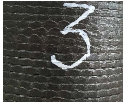
Figure 4.2. Welding surface M3: I_h=6.5\text{kA} ; F=2.3\text{kN} ; V_h=2.0\text{cm/s}
