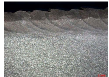
M3: I_h=6.5\text{kA} ; F=2.3\text{kN} ; V_h=2.0\text{cm/s}
