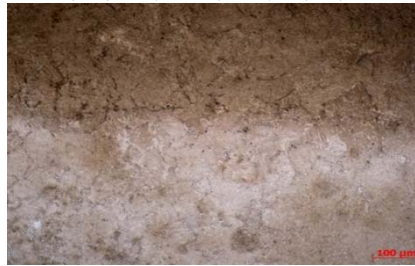
M5: I_h=7,5kA ; F=2,0kN ; V_h=2,0cm/s
