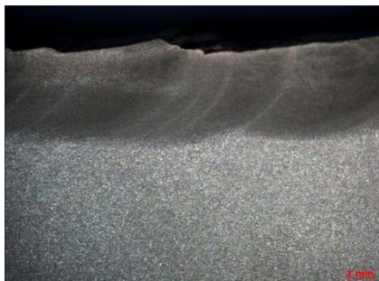
M7: I_h=8,5kA ; F=1,7kN ; V_h=2,0cm/s
